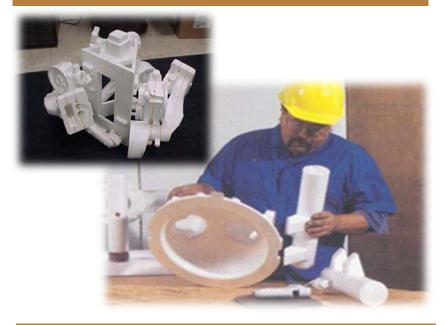
The moulded foam pattern can be a single pattern, several small patterns or a pattern in multiple sections.
