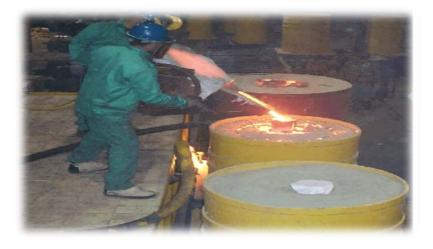
Before compaction the shell is placed into the flask and held in position by a fixture or by hand.
