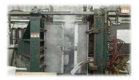
Foam Pattern Moulding on horizontal moulding machine
