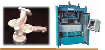
Foam Pattern Sections and Pattern Gluing Machine
