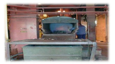
Casting is allowed to cool and solidify in sand for a predetermined period.
